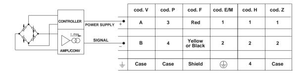
LOAD DIAGRAM (Current output)
